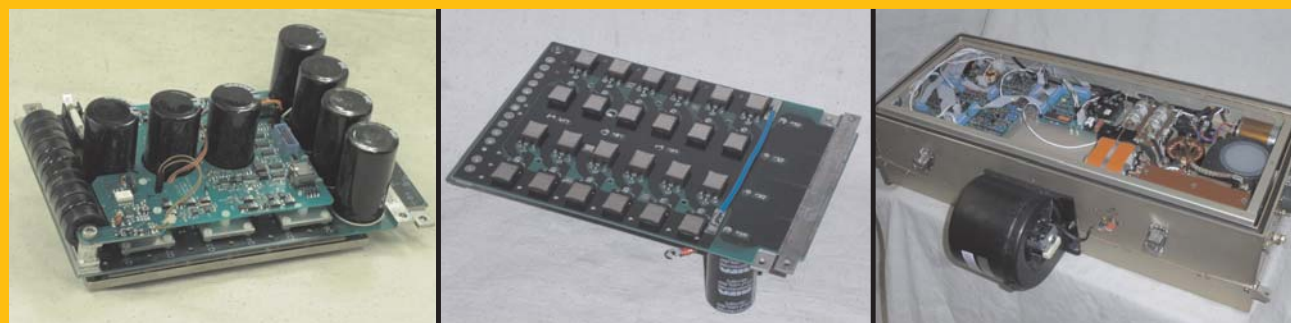
Fig. 10: AC Propulsion's Power Electronics Design. The three-phase motor drive is implemented with 12 parallel IGBTs in TO-247 packages for each of the switches, S1 - S6.
