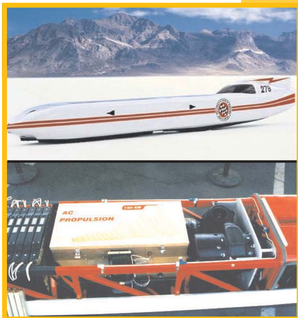
Fig. 13: dual AC Propulsion Drives powered this car to set the electric land speed record at 245.5 mph in October, 1999.
