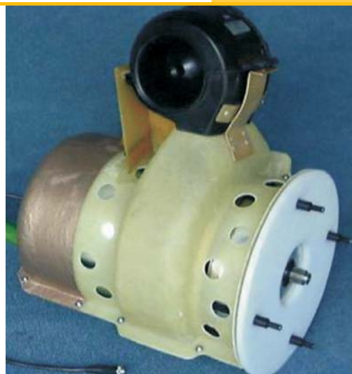
Fig. 11: AC Propulsion's 200 hp Traction Motor. Total weight is only 50 kg. and the motor is 90% efficient. The cost advantages of implementing this type of motor in place of a conventional gasoline engine are obvious.
